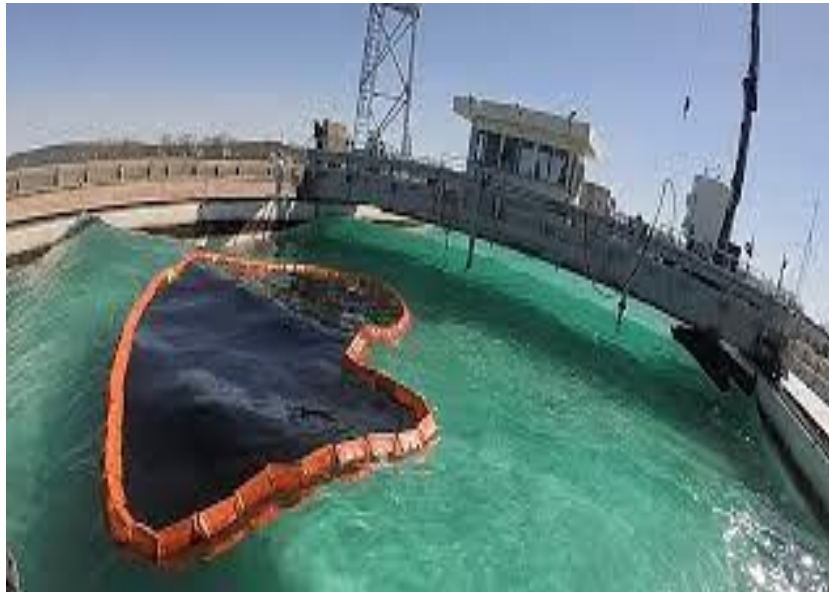
FIGURE 7 Harbo aims to be the first line of defense against oil spills with a floating barrier - or boom - that can be deployed in just 15 (Ariel Grossman, 2023)
