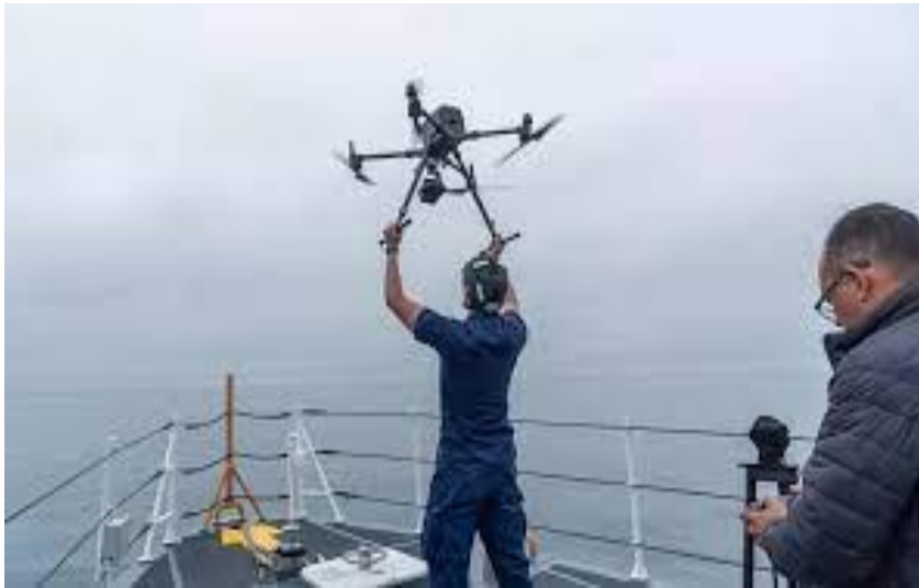
FIGURE 13 A crewmember of the Coast Guard cutter Blackfin releases a drone as part of Marine Oil Spill Thickness field campaign off the coast of Santa Barbara, CA . The drone carries a multi-spectral sensor to classify oil thickness. These data are compared with SAR imagery from NASA's aircraft UAWSAR . Oscar Garcia (right) of the Watermapping LLC controls the drone. Source: NASA/University of Maryland/Frank Monaldo
